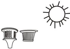
5. After drying, assemble the filter to the case
