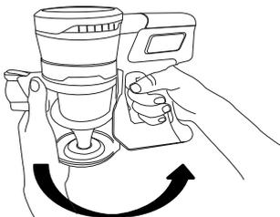
b) Attached the metal tube to the body as below until hear click sound
