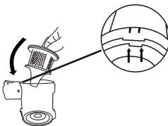
7. Assemble the dust cover into the dust cup as below showed
