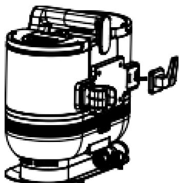
3. Remove the handle support and snap it onto the left-hand side of the rear cover.
