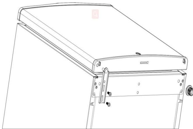
Step 4: Remove the top hinge and cover from right side to left side. Fasten the top door hinge with the screws, and cover the plastic cover and hinge cover.
