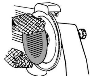
If the sliding carriage stops sliding smoothly, lay the machine on its side.
