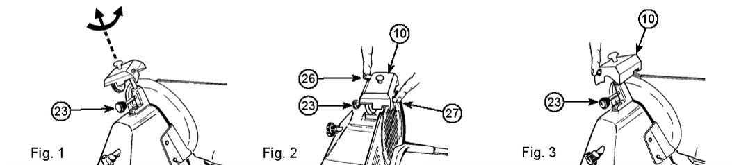
N.B.: it should be noted that the blade is highly resistant, therefore it needs to be sharpened only when the capacity of cut decreases. The gauge plate or guard plate shall be closed on slicers with an integral blade sharpener during the sharpening operation.
