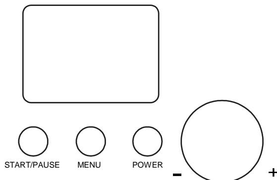
**[POWER]** : After powering up, the machine enters standby mode. Then press the **[POWER]** button to enter the setting mode, and LCD will display “60 : 00”. Press the **[POWER]** button during setting mode, the machine will enter the standby mode again.
