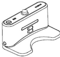
Station de charge
