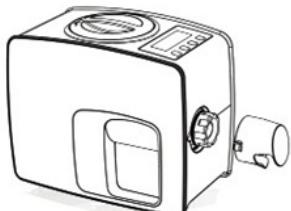
3. Unscrew the extrusion shaft with the special spanner included in the box, in a counterclockwise direction and then take out the outer part.
