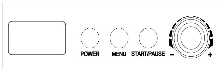
**[POWER]:** After power up, the machine enters standby mode. Then press the **[POWER]** button to enter the setting mode, and LCD will display "60: 00" and light up the background light. If no other operation, the light will go off 15 seconds later; then press the **[POWER]** button again; the machine can go back to standby mode.
