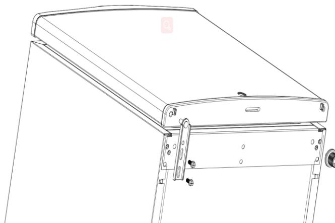
**Step 4:** Remove the top hing and cover from right side to left side. Fasten the top door hinge with the screws, and cover the plastic cover and hinge cover.
