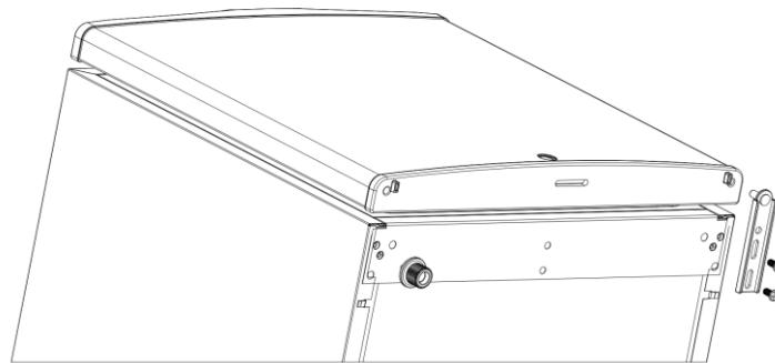
Step 3 : Displace and fasten the bottom door hinge including the feet with the screws.
