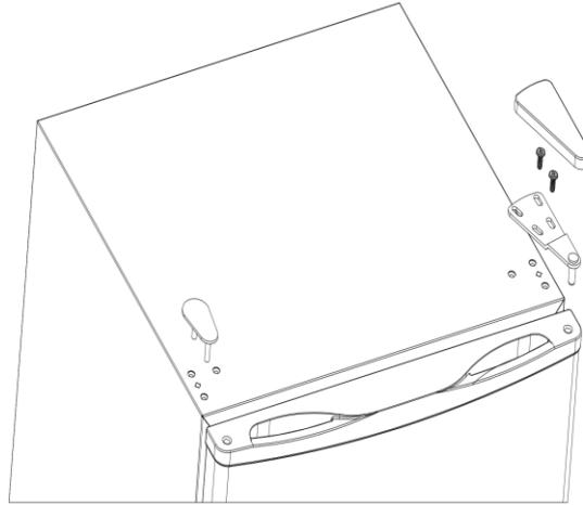
Step 2 : Disassemble the lower door hinge and the feet by loosening the screws.
