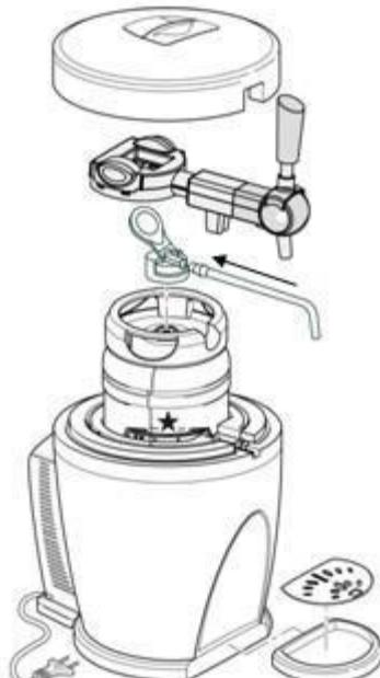
3. When the ambient temperature is 25°C and the HeineKen keg is placed, power the unit up with DC current or AC current for 48H, the beer temp will up to and maintain 3~6°C.(3°C means the cooler is running, 6°C means it is
