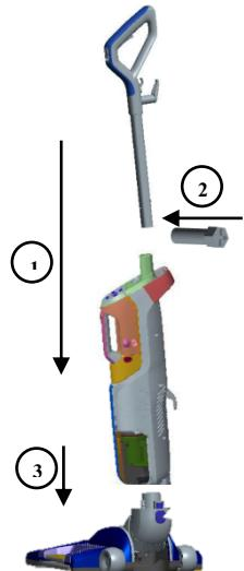
1. Insert the end of handle assembly into the main body
