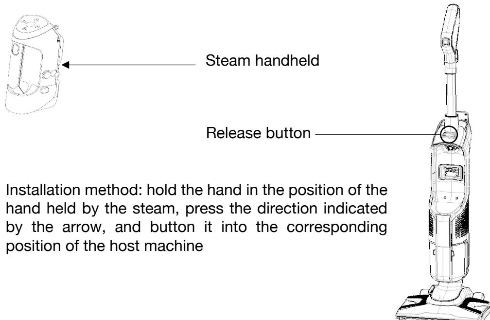
Installation method: hold the hand in the position of the hand held by the steam, press the direction indicated by the arrow, and button it into the corresponding position of the host machine
